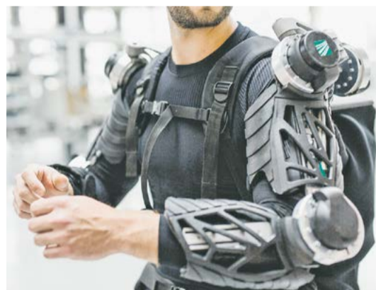
The Exo Jacket offers workers support during lifting tasks and overhead work, allowing them to stay healthier and work longer – a relevant benefit in view of the ageing workforce. Photo: Ludmilla Parsyuk / Fraunhofer IPA
